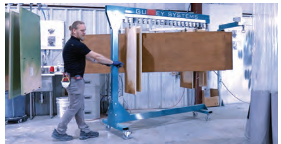
By using multiple mobile rails, Oldwood Custom Cabinets is able to continuously move parts in and out of the spray area while dramatically reducing material handling and increasing volume.
