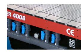
The vacuum deck can be configured with either standard vacuum zones or they can be customized for specific requirements and part sizes.
