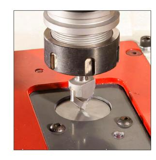
The tool-length sensor is used to automatically measure the length of a tool and create an accurate tool-length offset. This time-saving feature also ensures precise and consistent cutting depths with all tools
