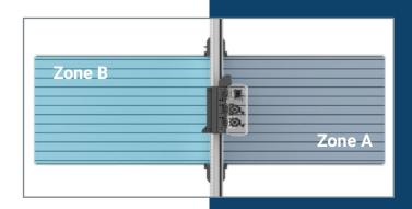
Pendulum processing allows truly continuous production by splitting the process area into two virtual zones so that a sheet can be processed on one zone while parts and waste from the other are removed.
