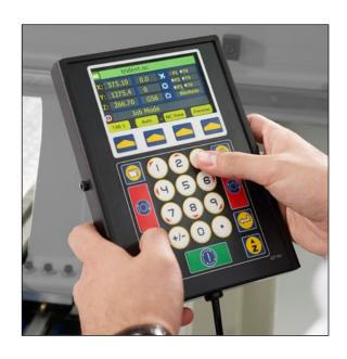
The AXYZ SmartConsole brings unprecedented ease of use, context sensitive menus, real-time display of machine status and many more time-saving, functional and productivity features. It provides a graphical preview and current status of a running job and allows program feeds and speeds to be changed without pausing the program.
