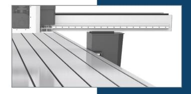
For applications that need a greater vertical clearance such as mold making or three dimensional carving, the standard 6" (150mm) gantry height can be extended to 10" (250mm), 12" (300mm) or even greater.
