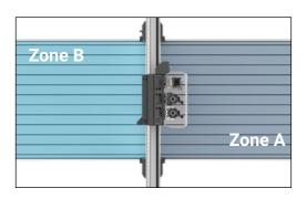
Pendulum Processing mode allows continuous production on two virtual beds. Eliminate machine downtime in between jobs to achieve up to twice the productivity.
