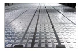
The innovative design of the aluminum vacuum deck allows zoned areas to be opened or closed as needed. Flat sheet materials are held as securely as possible while cutting problems caused by movement or vibration of the materials are virtually eliminated.
