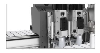
Choose a single, double or even triple-head configuration for applications that typically require multi-tool cutting operations. A twin carriage option is also available, enabling you to copy cut two parts at the same time, effectively doubling production capacity and enabling a faster turnaround on jobs.
